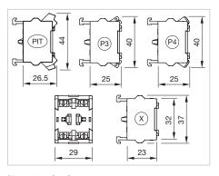
Dimensions [mm] PIT = Push-in terminal, P3 = Plug-in terminal 6.3 x 0.8 mm, P4 = Double plug-in terminal 6.3 x 0.8 mm, X = Screw terminal
